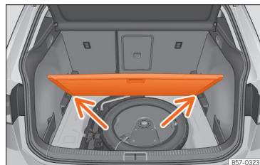
Fig. 174 Variable boot floor: tilted position.
