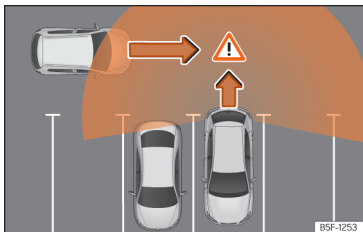
Fig. 154 Diagram of the parking assistant: detected area around the vehicle that is driving off.
