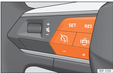
Fig. 114 On the multifunction steering wheel: cruise control operation buttons.
