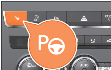
Fig. 141 In the centre console, top section: button to switch on the Park Assist system.
