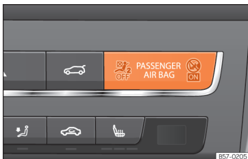
Fig. 30 Dashboard: control lamp for deactivated front passenger airbag in centre console.
