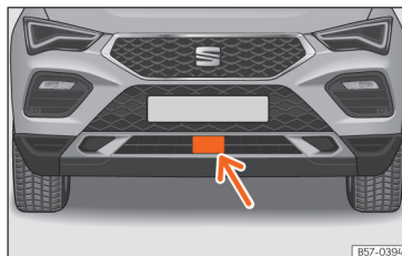
Fig. 108 On the front bumper: radar sensor.
