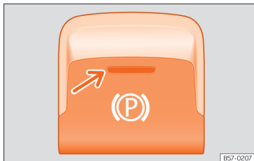
Fig. 134 Centre console, lower part: electronic parking brake button.
