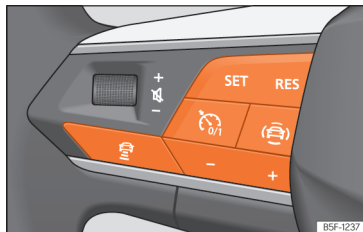
Fig. 118 On the multifunction steering wheel: buttons for operating the ACC.
