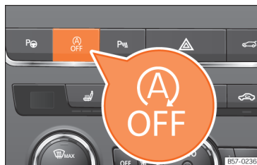
Fig. 99 Centre console: Start-Stop system button.
