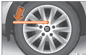
Fig. 226 Tyre change: slacken the wheel bolts.
