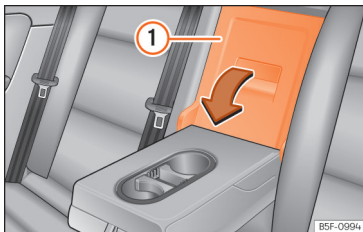
Fig. 180 On the rear seat backrest: opening the tailboard.
