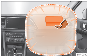
Fig. 28 Front passenger airbag located in dash panel.
