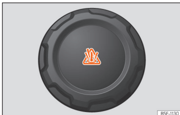
Fig. 210 Front compartment: coolant expansion tank cap.
