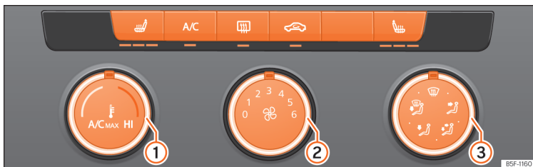
Fig. 93 In the centre console: manual air conditioning control panel.
