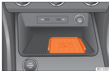
Fig. 168 On the centre console: pad for the mobile phone connection.
