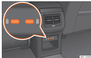
Fig. 161 Rear centre console: USB connectors with power socket function.
