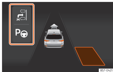
Fig. 142 On the instrument panel display: display of the assisted parking system with decreased visibility.
