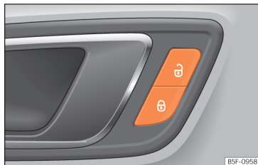
Fig. 54 On the driver's door: central locking system button.
