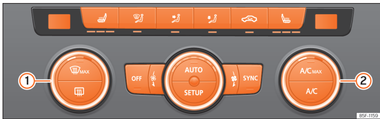
Fig. 92 On the centre console: Climatronic controls.
