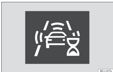
Fig. 125 On the instrument cluster screen: indication of the system's initial self-calibration.
