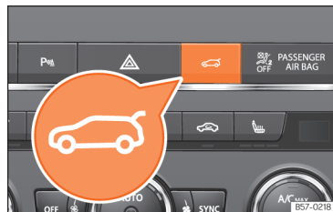
Fig. 61 Centre console: button to open and close the rear lid.
