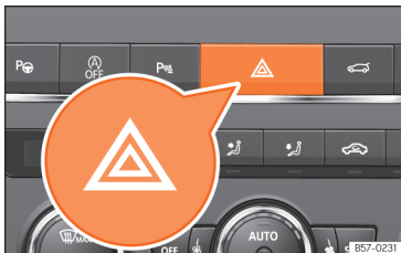
Fig. 44 Dashboard: switch for hazard warning lights.
