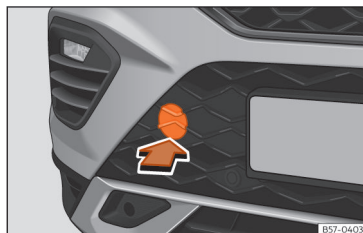
Fig. 197 Front bumper on right: remove the lid.
